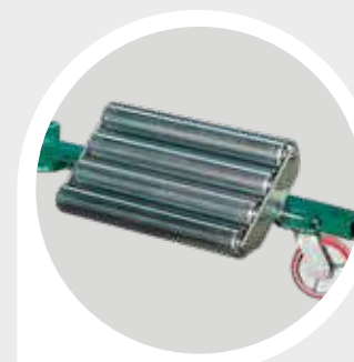
2 x 4 large rollers improve handling of tyres with deep treads.
