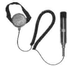
Pedal force sensor
