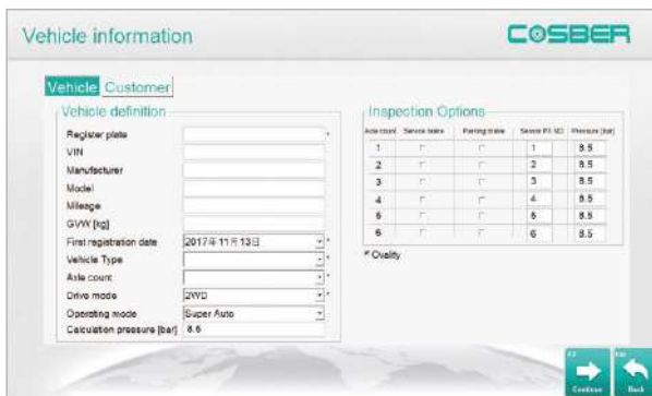
Configuration of axles and air-pressure sensor
