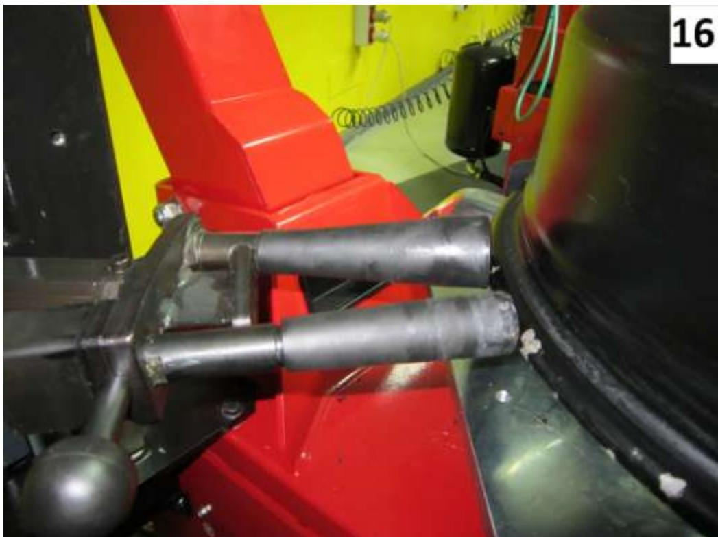
2. Make sure that the rollers are tangential to the rim (IMG 17);
