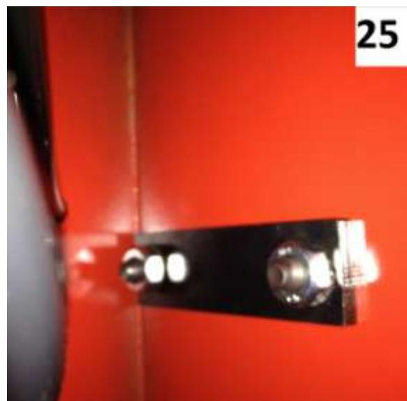
6. Tighten the screw, toothed washer and nut to fix the bottom part of the UPH to the body (IMG 5 and IMG 6);
