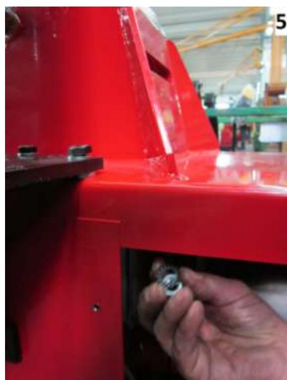
3. Position the 3 screws M10 x 30 as showed in the picture IMG 23;
