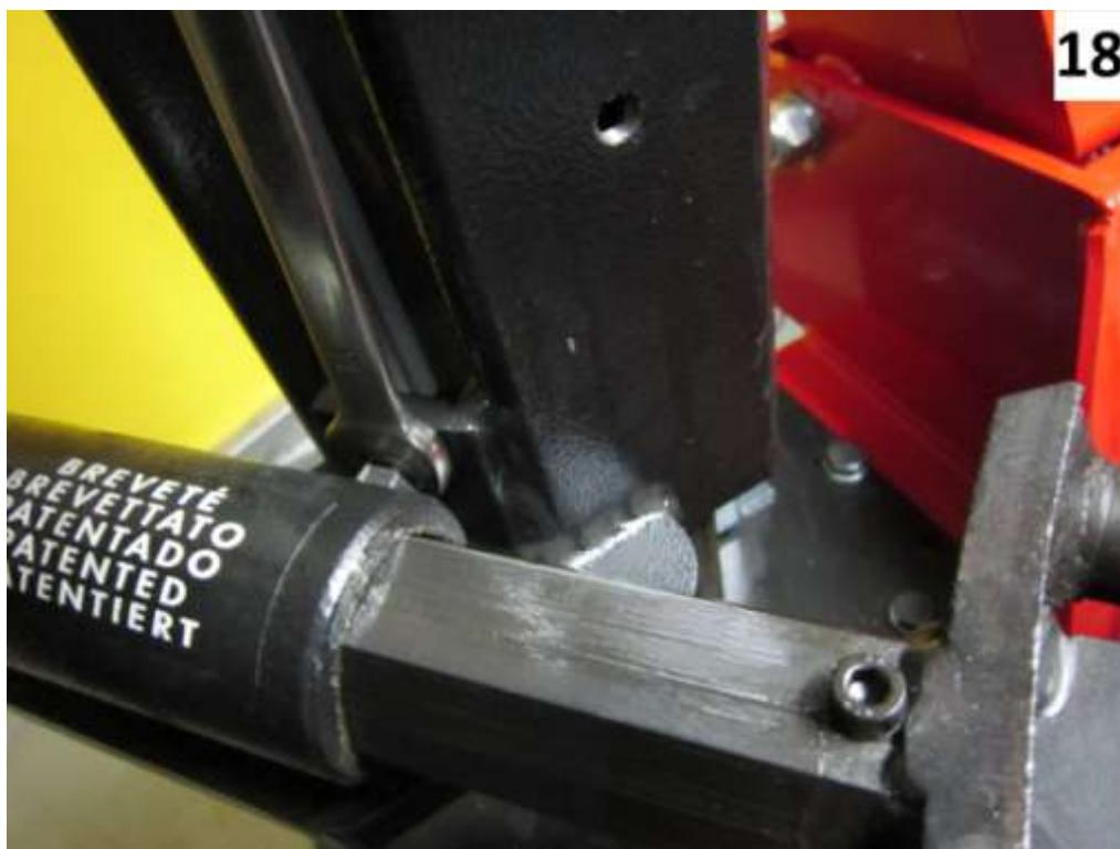
4. Lead the UPH fork towards the upper edge of the rim and check the distance: fixed roller – rim edge (it must be 2 mm approx.) (IMG 19);
