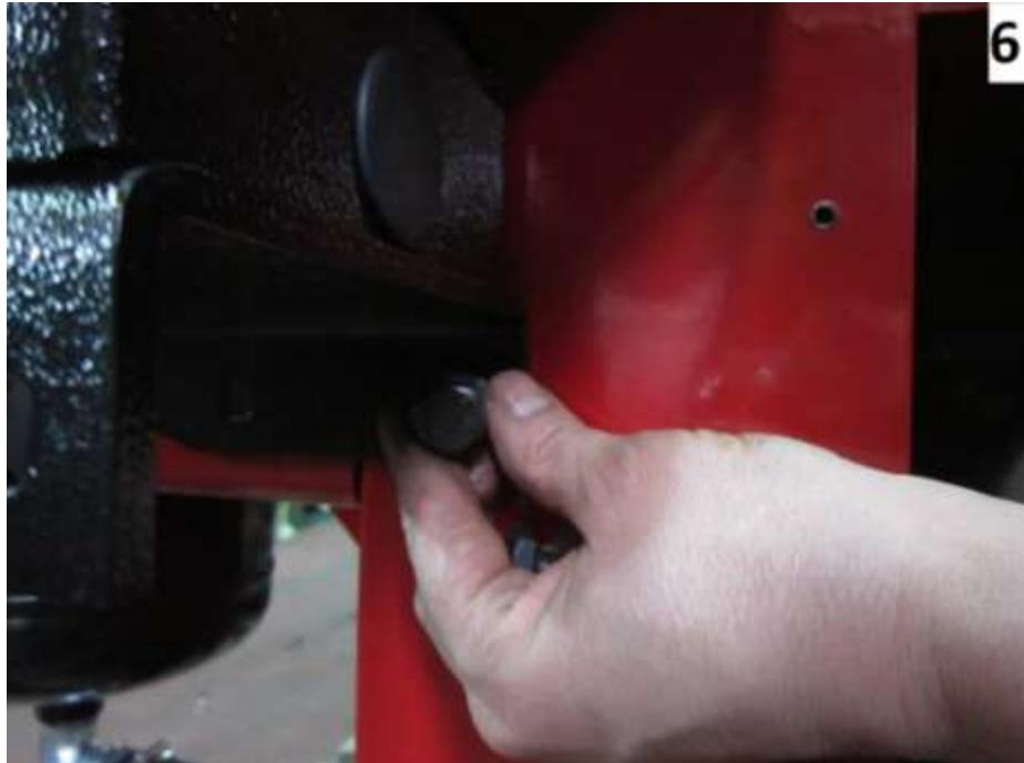
7. Tighten the screw, washer, toothed washer and nut to fix the lateral part of the UPH to the body (IMG 23)
