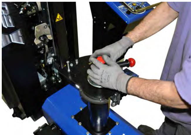
Install the calibration jig on clamping chuck
