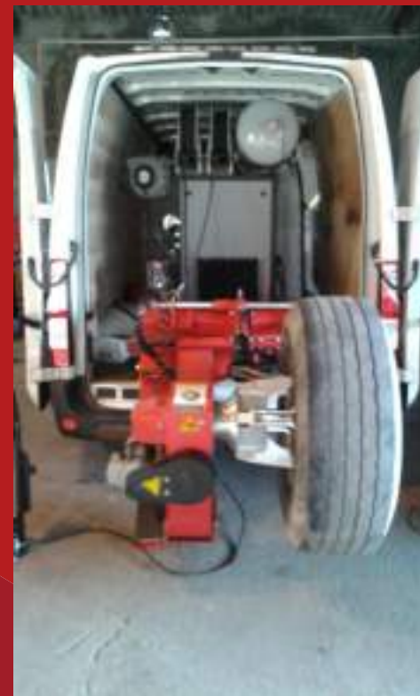
INSTALLATION AT REAR DOOR WITH INVERTED CHUCK
