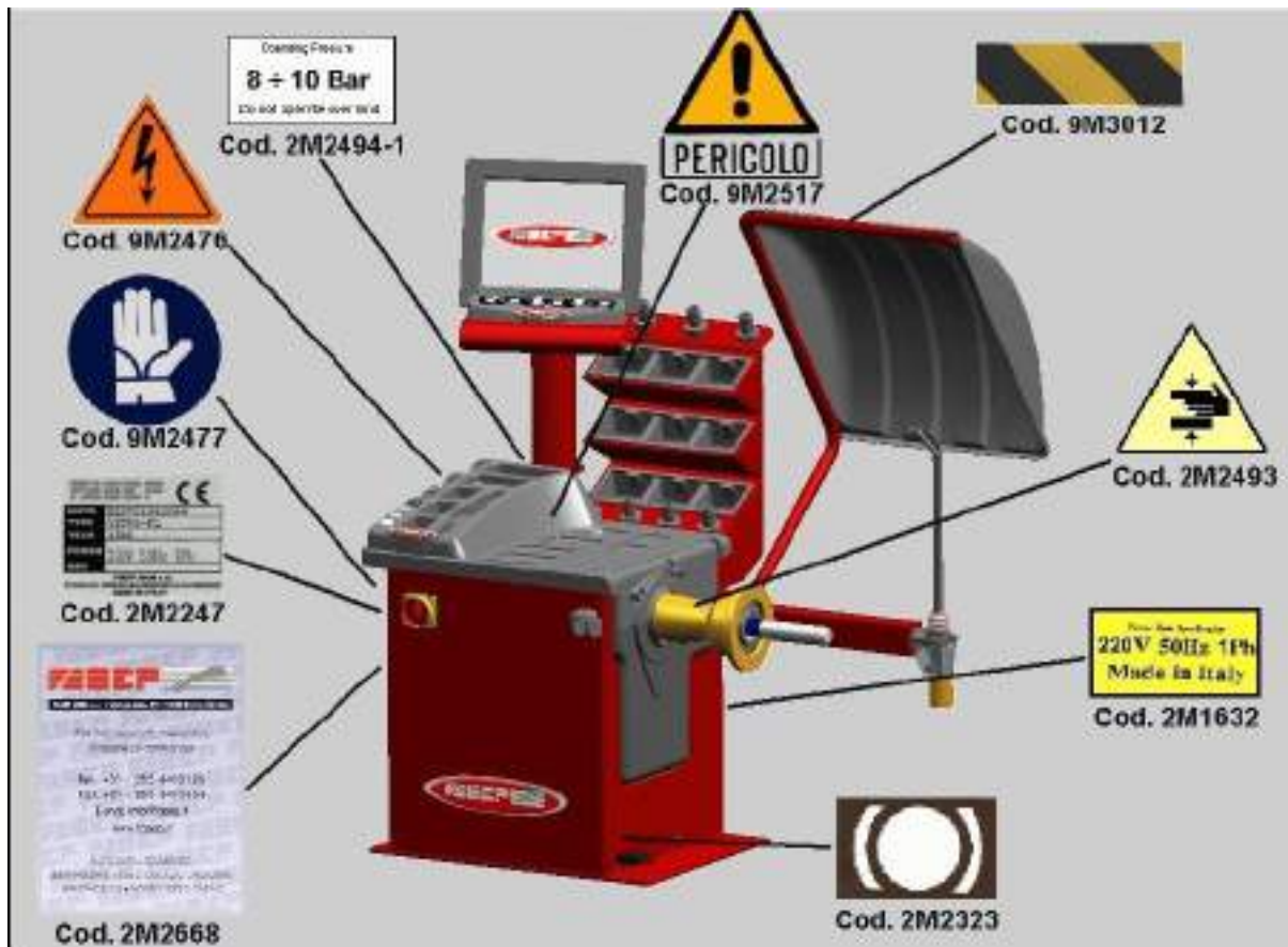
Fig. 75 Labels applied to wheel balancer
