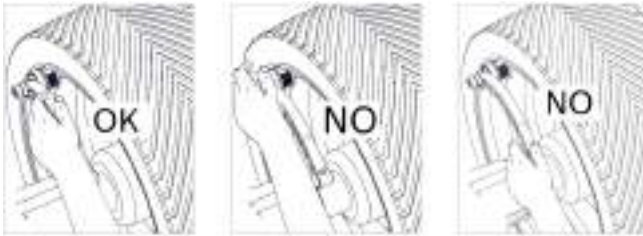
Fig. 28: Correct handling of the electronic rim distance gauge
