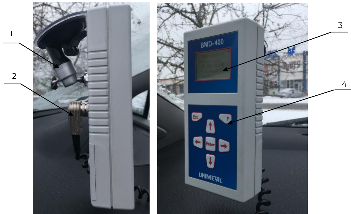
Fig. 9 – BMD-400 device mounted on a vehicle windscreen; 1 – Handle, 2 – Plug of brake pedal pressure meter, 3 – Display, 4 – Keyboard
