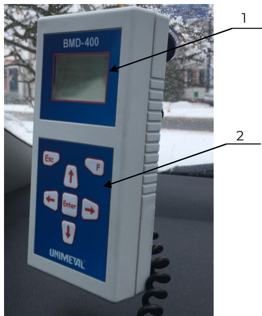
Fig. 1 – BMD-400 device; 1 – LCD screen, 2 – buttons
