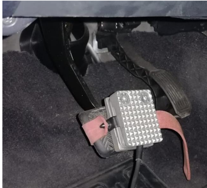
Fig. 10 – Brake pedal force transducer installed on a brake pedal
