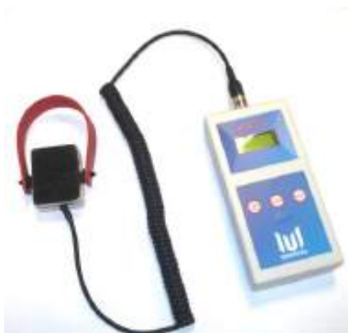
Fig. 5 – Effort meter for brake pedal connected to the measuring device BMS-100
