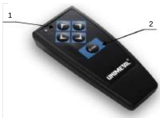
Fig. 8 – Remote control; 1- navigation buttons, 2- confirm button
