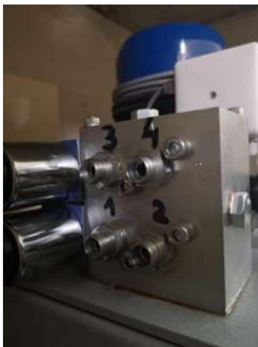
Fig. 18 - Hydraulic power supply cube
