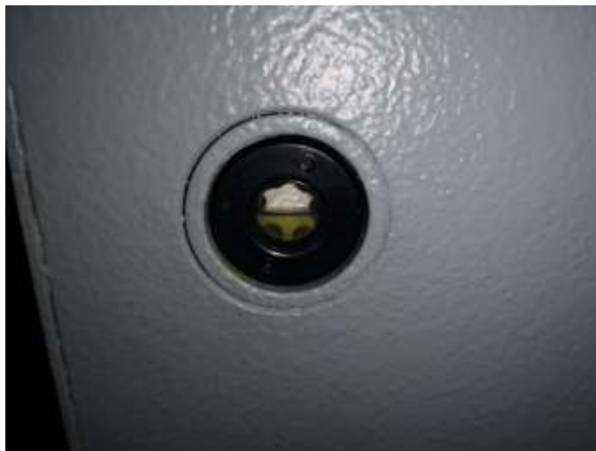
Fig. 24 - Window in the hydraulic power supply for checking the oil level.
