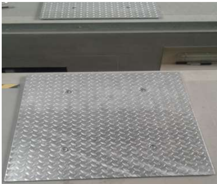
Fig. 17 - SZ-16 device with moving plate mounted in foundation
