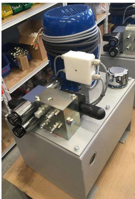
Fig. 3 – Hydraulic power supply
